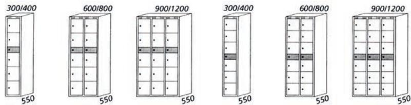
Cabinet height without legs: Flat top 1740 mm and sloping top 1940 mm. Depth 550 mm.
