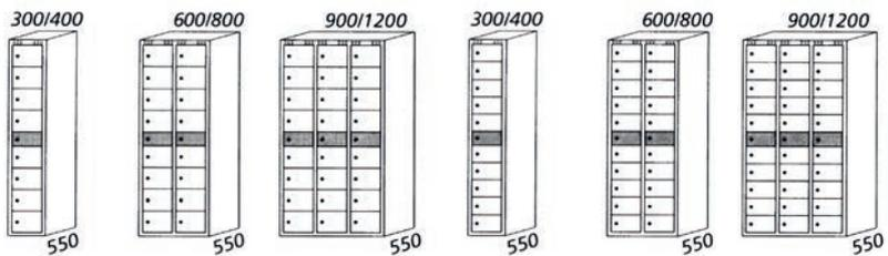
Cabinet height without legs: Flat top 1740 mm and sloping top 1940 mm. Depth 550 mm.
