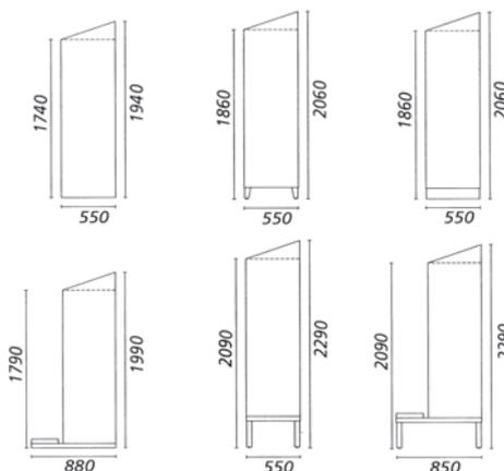
Model GDTS (sloping top) is 2 cm lower on the back edge and 5 cm less deep than GS.
